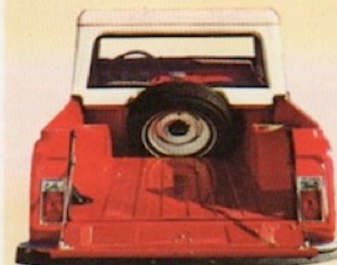
Spare tire is mounted to allow full use of cargo area, yet permit driver's unobstructed view through rear window.
